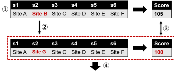
Fig. 3. Hill Climbing ( n = 6 ). ①:Initialization ②:Generation of neighboring solutions ③:Solution update by selecting the better one ④:Iteration
